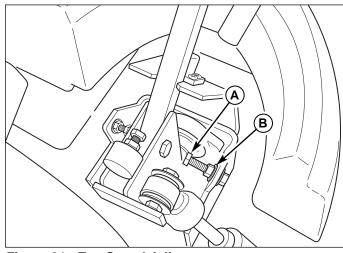
Figure 31. Top Speed Adjustment
